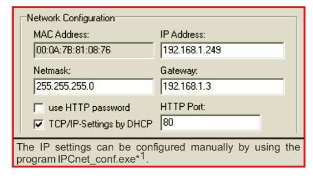
Start the IPower Control in boot mode (see section 7) and launch the IPCnet\_conf.exe program. The program will automatically search for connected devices and display their IP settings. If displayed address the IΡ matches the default setting (192.168.0.2) there is either no DHCP server available or no unused IP address could be allocated.
